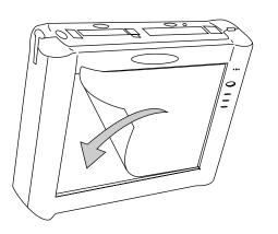
Figure 6. Applying the Screen Protector
